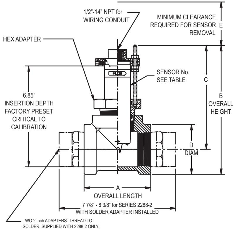
NOTE - DIMENSIONS "8" AND "C" MAY VARY +/- 1/4 inch. DEPENDING UPON MAKE-UP ON PIPE THREADS>
